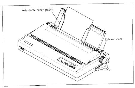
Figure 3-5. Place a single sheet between the guides.
