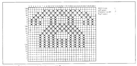
Figure 9-2. Telephone symbol with normal LQ pica.
