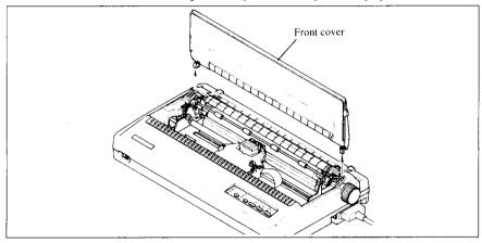
Figure 7-2. Remove the front cover from the printer.
