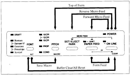
Figure 4-2. Switch combination functions of control panel.
