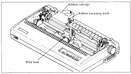
Figure 2-5. Install the ribbon cartridge.
