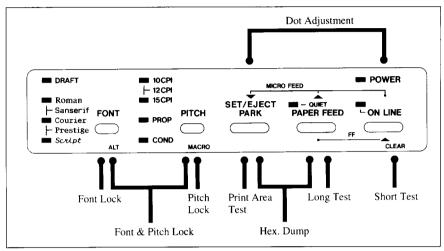
Figure 4-3. Power-up functions of control panel.
