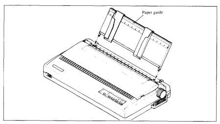
Figure 2-8. Install the paper guide.
