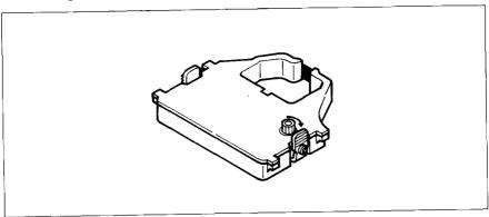
Figure 2-4. Take up the slack in the ribbon by turning the tension knob on the ribbon cartridge.
