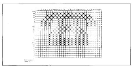
Figure 9-3. Telephone symbol with LQ pica.
