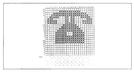
Figure 9-5. Compressed character pattern of telephone symbol.
