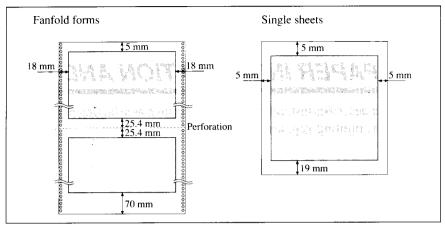
Figure 3-1. Recommended print area for acceptable types of paper.
