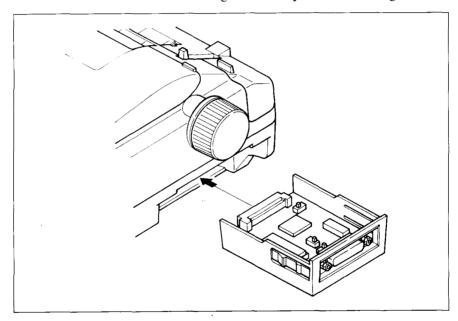
Figure 7-17. Replace the interface cartridge.
