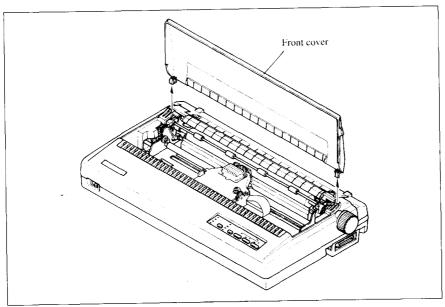
Figure 2-3. Remove the front cover to install the ribbon cartridge.
