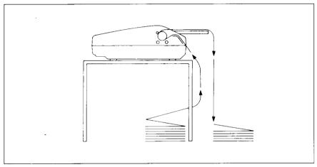
Figure 3-6. Paper path for fanfold forms.
