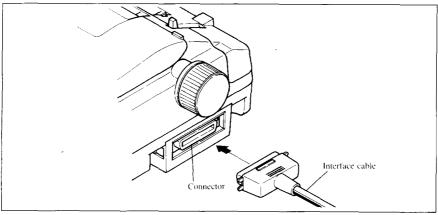
Figure 2-9. Connect the interface cable.
