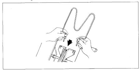
Figure 7-5. Insert the hopper attachment.
