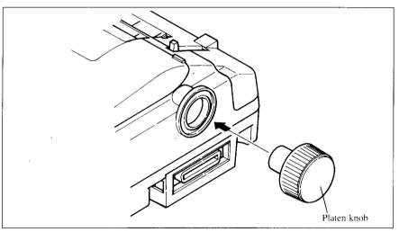
Figure 2-2. Installing the platen knob.
