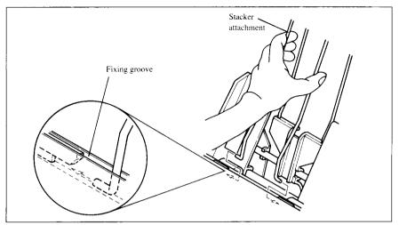
Figure 7-6. Insert the stacker attachment.
