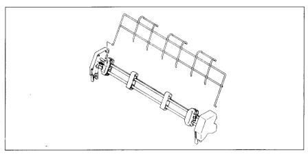
Figure 7-11. Attach the paper support to the pull tractor.
