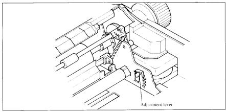
Figure 3-2. Location of the adjustment lever.
