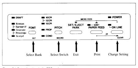
Figure 5-1. Button functions in the EDS mode.
