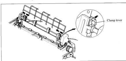
Figure 7-14. Adjust the sprocket guides.
